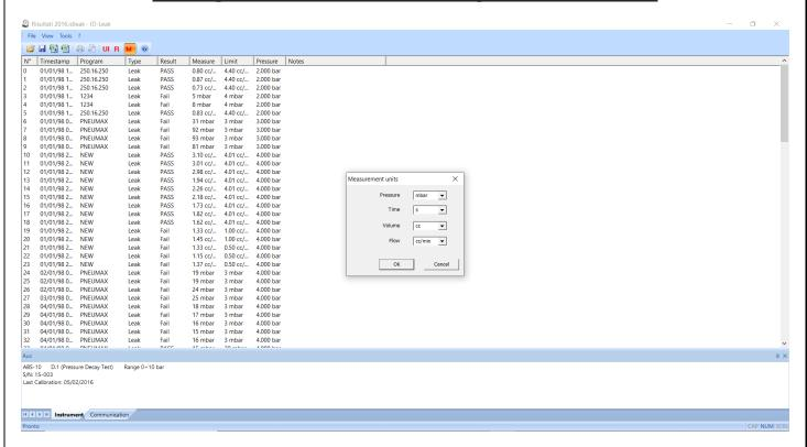
ID-Leak software allows you to download, save and manage the results of leak tests carried out with a SMARTLEAK device.
